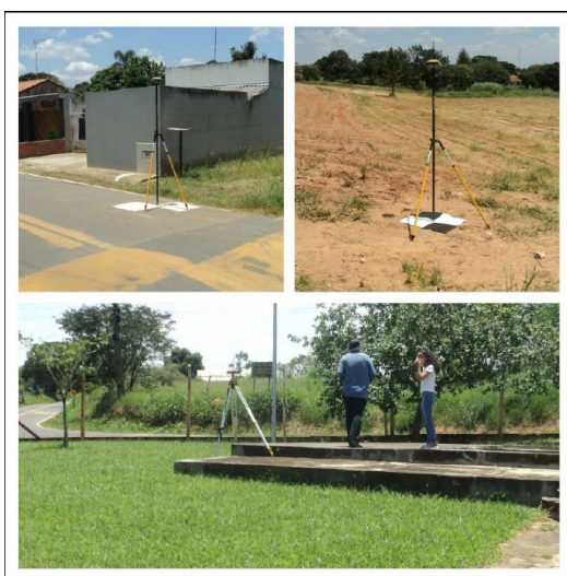
Figure 6 – Allocation of the geodetic GNSS base station and collection of control points with the survey station. Source: Authors (2022).
