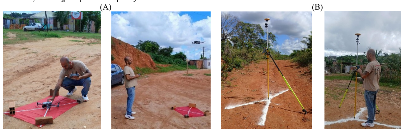
Figure 3. (a) Photogrammetric survey; (b) Check point acquisition.
