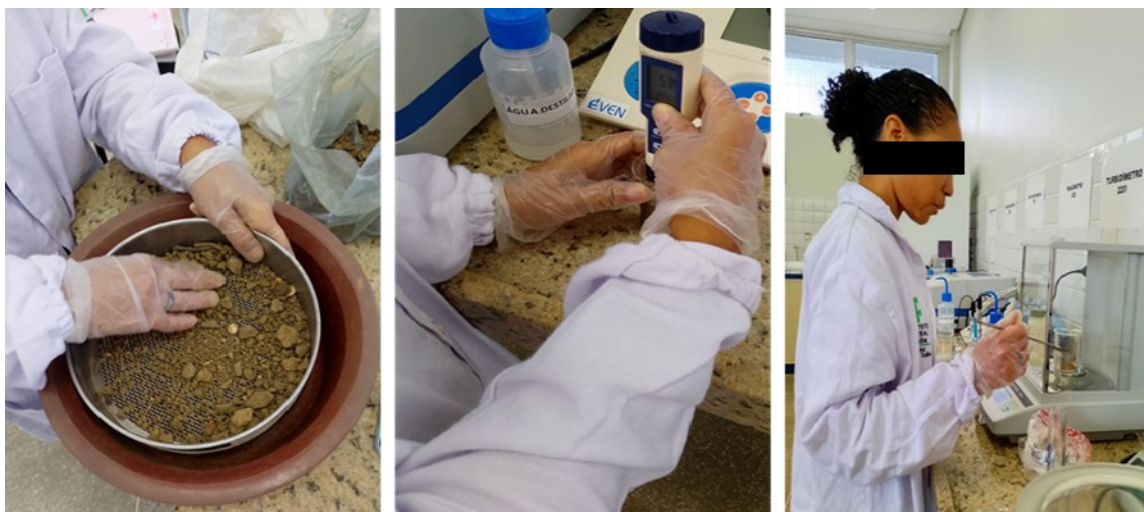
Figure 4 – Sieving, pH measurement, and weighing procedures.
