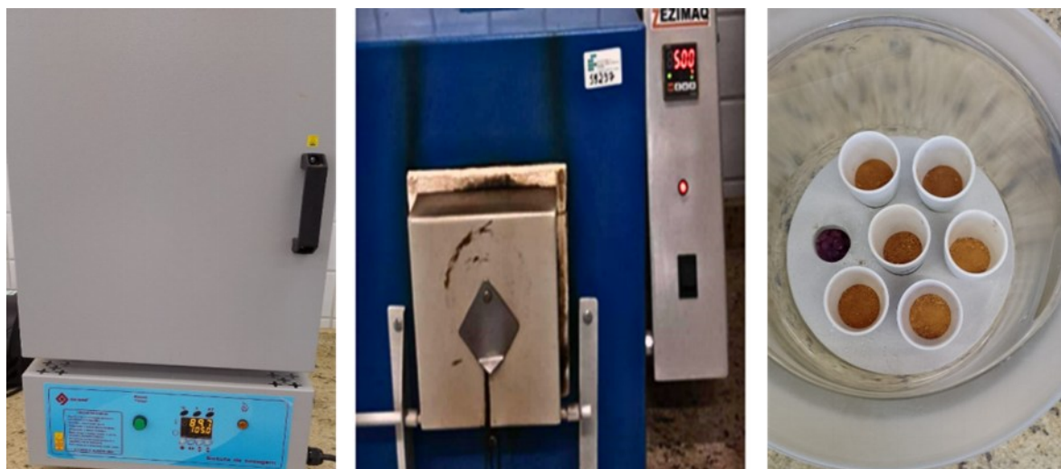
Figure 3 – SOM determination process. Source: Authors (2025).
