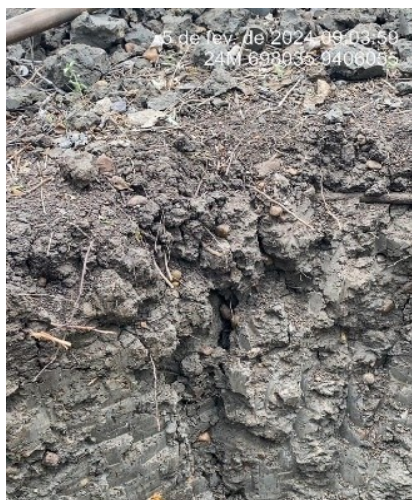
Figure 3 – Expansive soil profile of the Mossoró/RN region. Source: Braz (2024).
