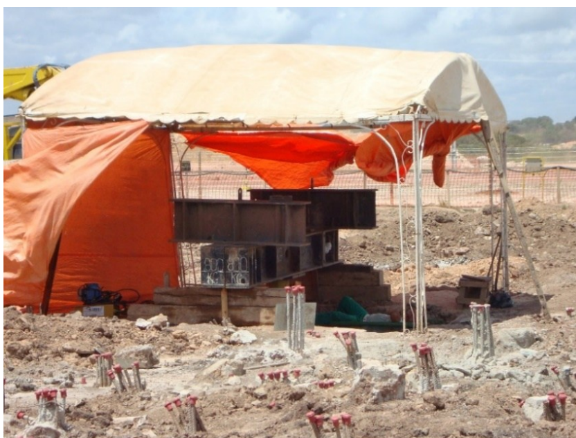
Figure 18 – Structure assembled to perform the load test at Petroquímica Suape. Source: Adapted from COUTINHO (2008).
