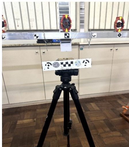
Figure 3 – Distribution of photogrammetric targets for control points and object points. Source: Authors (2024).
