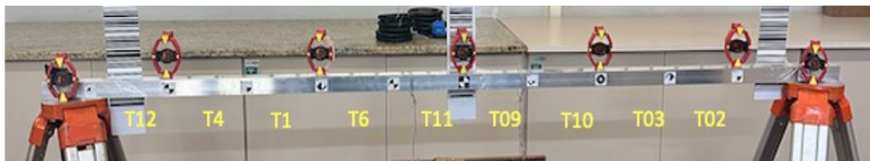
Figure 10 – Arrangement of targets used for the photogrammetric process.
