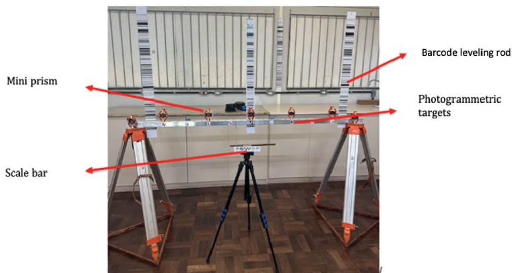
Figure 1 – Arrangement of the study object and targets used in measurements. Source: Authors (2024).
