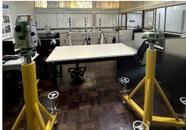
Figure 2 – TS15 ETR and DNA03 Level installed on industrial tripods. Source: Authors (2024).
