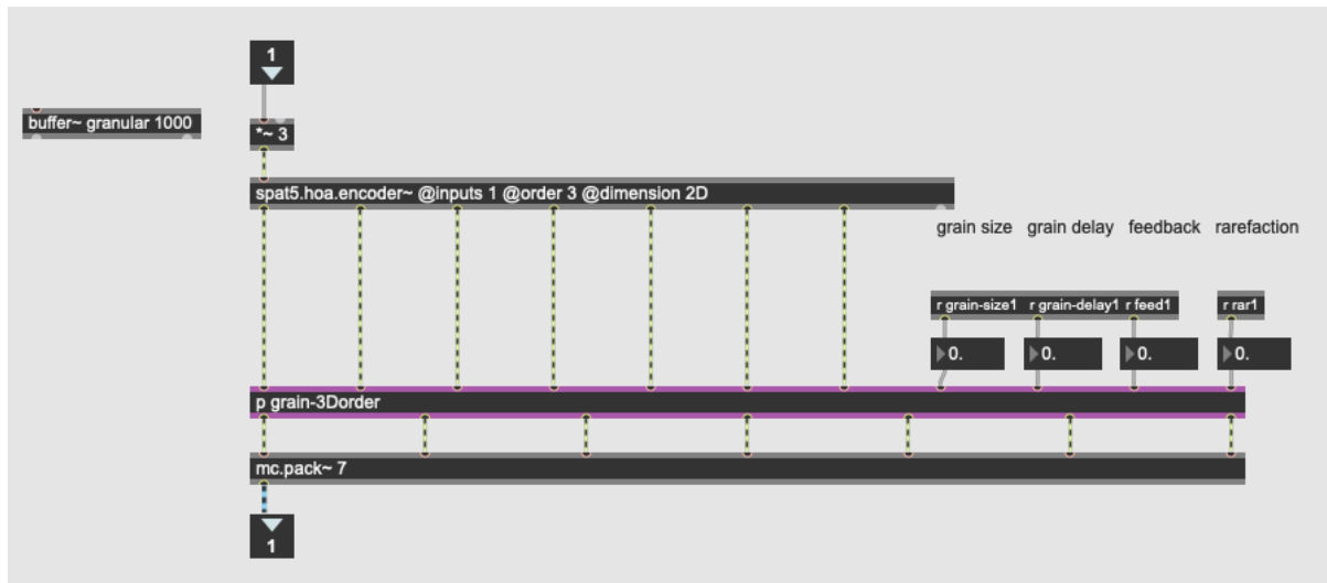
Figure 3 – Subpatch of granular synthesis applied to flute sounds, located between the encoding and decoding processes in ambisonics
